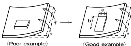
(2) Components location on PCB separation
