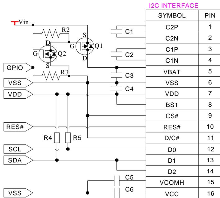
**Recommended Components:**C1, C2: 1 $\mu$ F / 16V, X5RC3, C4: 1 $\mu$ F / 16V, X5RC5, C6: 4.7 $\mu$ F / 25VR2, R3: 47k $\Omega$ R4, R5: 4.7k $\Omega$
