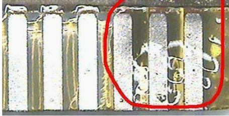
A photograph of several PCB pins. One pin is circled in red, showing a white, irregular substance (glue or contamination) that has hardened on its surface.                                          |
