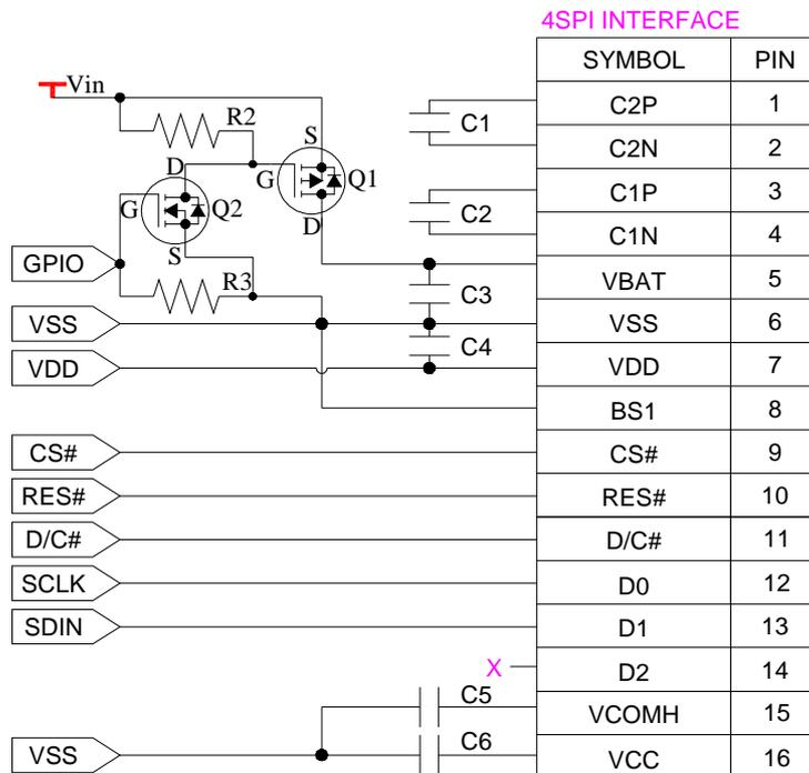
**Recommended Components:**C1, C2: 1 $\mu$ F / 16V, X5RC3, C4: 1 $\mu$ F / 16V, X5RC5, C6: 4.7 $\mu$ F / 25VR2, R3: 47k $\Omega$
