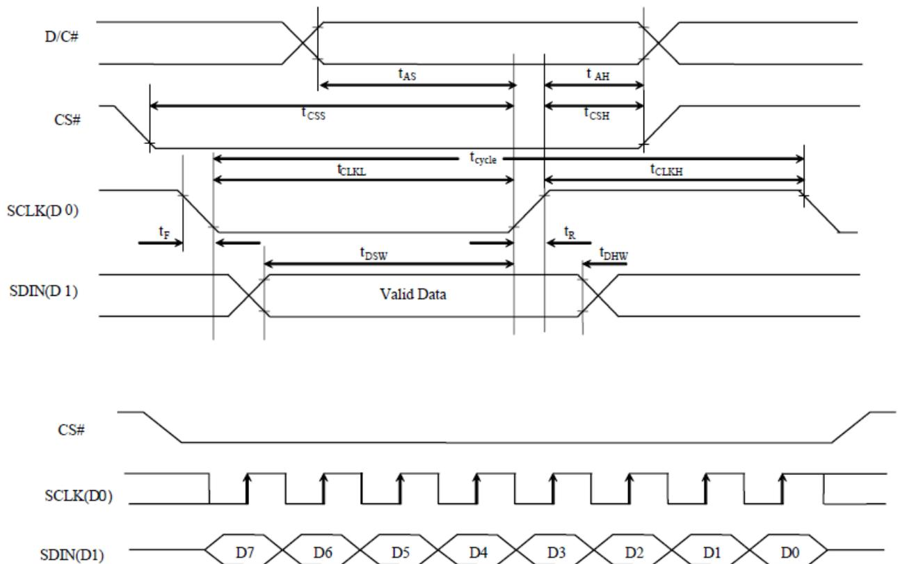
9-3-2 I<sup>2</sup>C Interface Timing Characteristics
