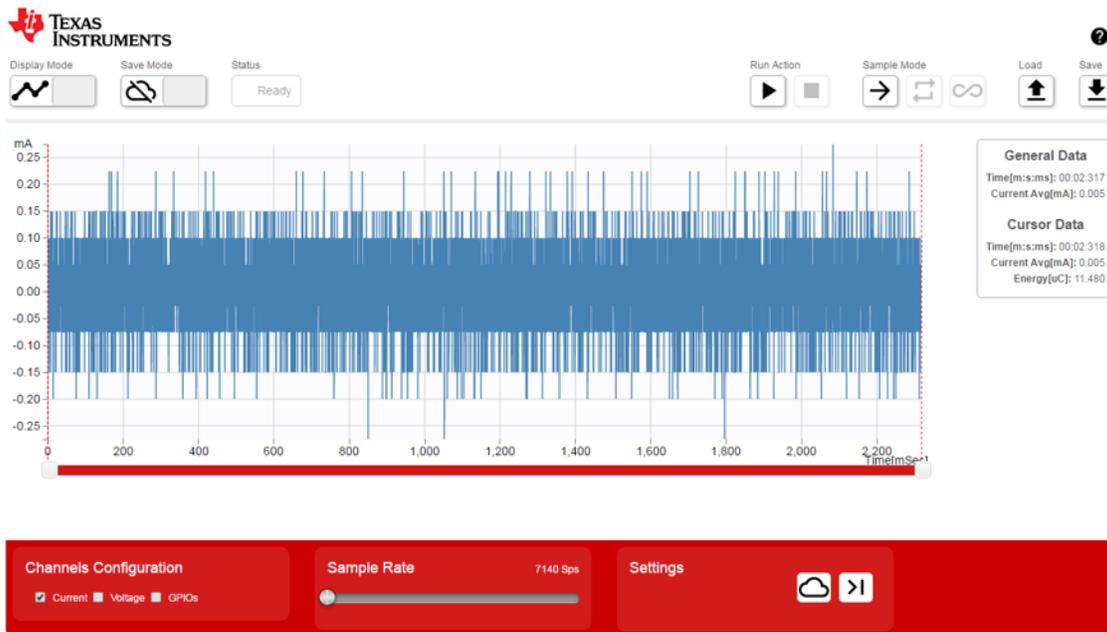
Figure 16. Wireless Scope Measurement of CC3100 Hibernate
