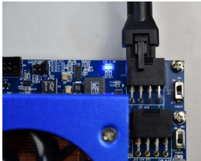
Figure 1-10 Connect 12V ATX Power Connector to Apollo S10
