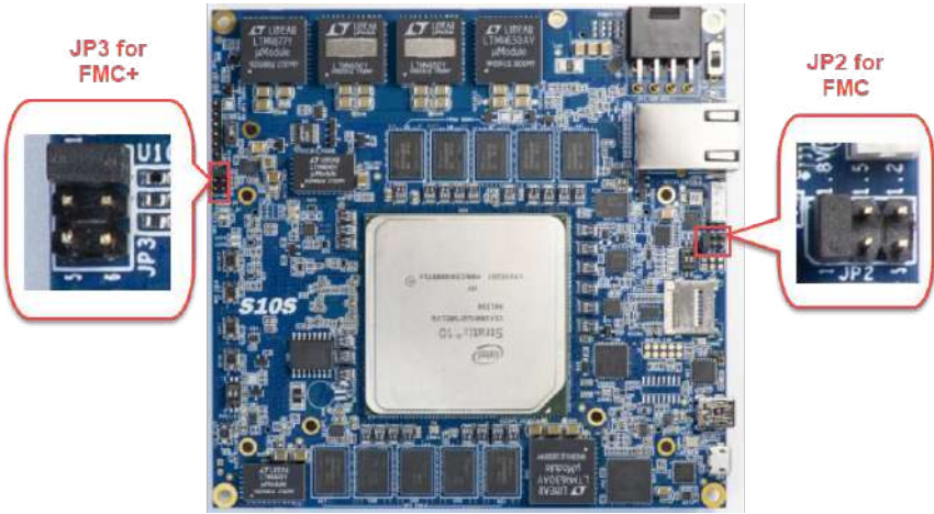
Figure 2-6 FMC and FMC+ I/O standard setting headers
