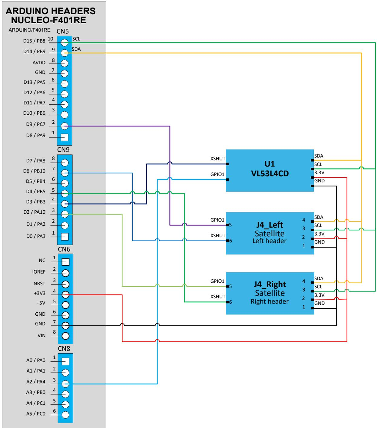
Figure 5. VL53L4CD-SATEL simplified schematic
