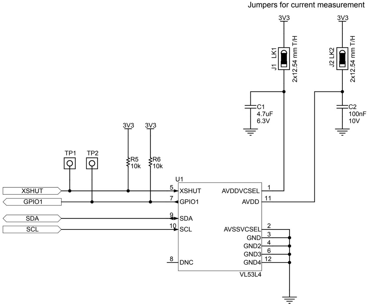
**Figure 8. X-NUCLEO-53L4A1 circuit schematic (3 of 6)**
