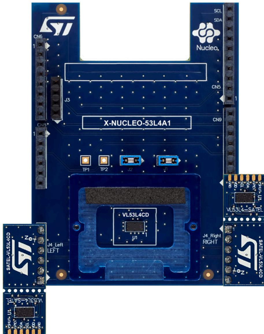
**Figure 3.** VL53L4CD mini PCB flying wires connection to X-NUCLEO-53L4A1 expansion board
