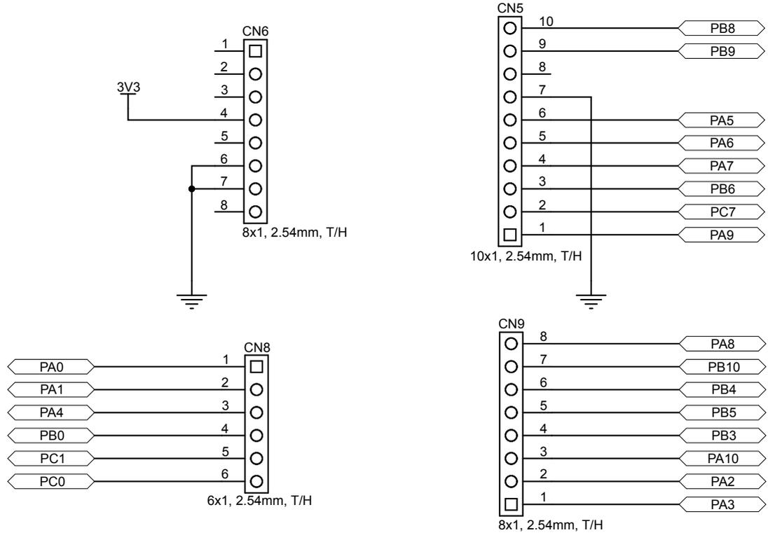
**Figure 9. X-NUCLEO-53L4A1 circuit schematic (4 of 6)**
