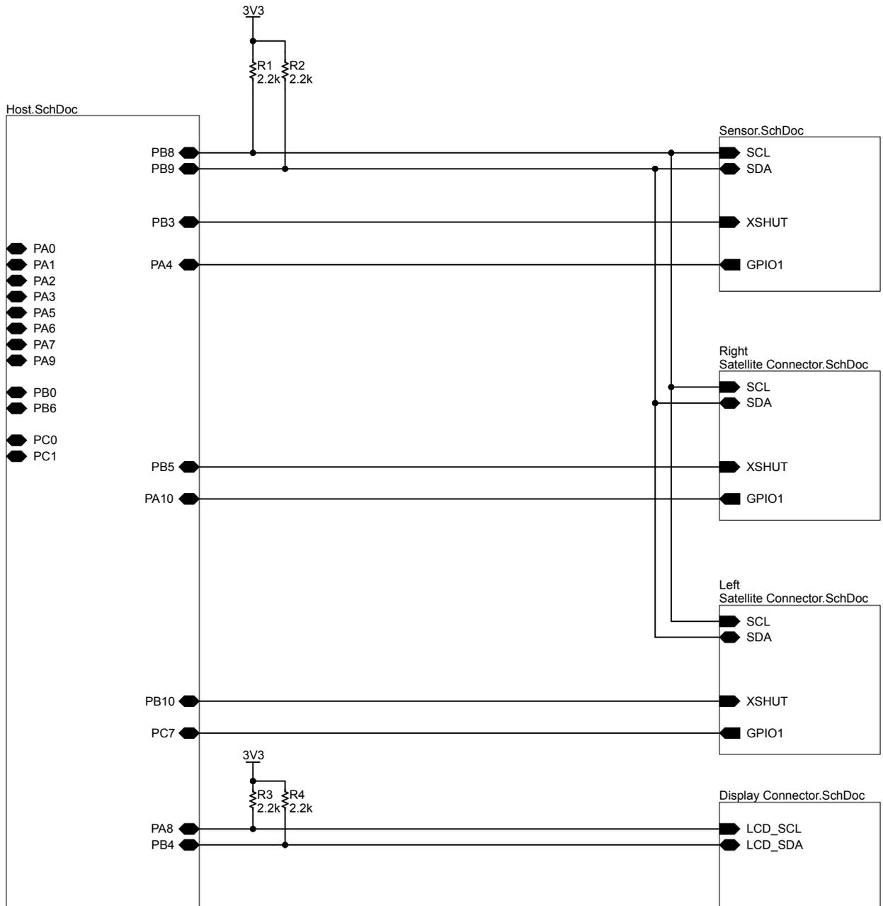
Note: The display connector is an optional connector to connect an SSD1306 I2C OLED display to output the ranging data or other meaningful information if required. The related application note and example code will be available on [st.com](http://st.com).
