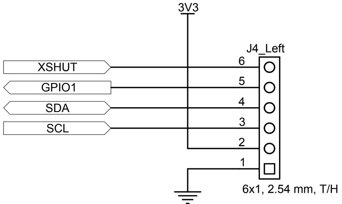
Figure 11. X-NUCLEO-53L4A1 circuit schematic (6 of 6)
