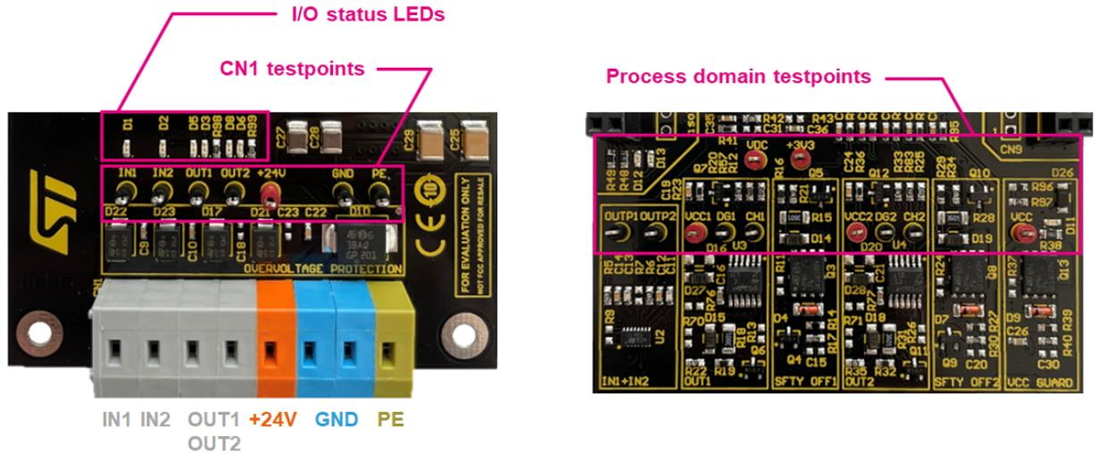
To allow easy system function testing and laboratory measurements the **STEVAL-FSM01M1** contains a set of onboard testpoints which provide measuring access to all the key voltage nodes in the system (power supply voltage, logic section supply and digital I/O status and diagnostics). These testpoints are also shown in **Figure 3**.
