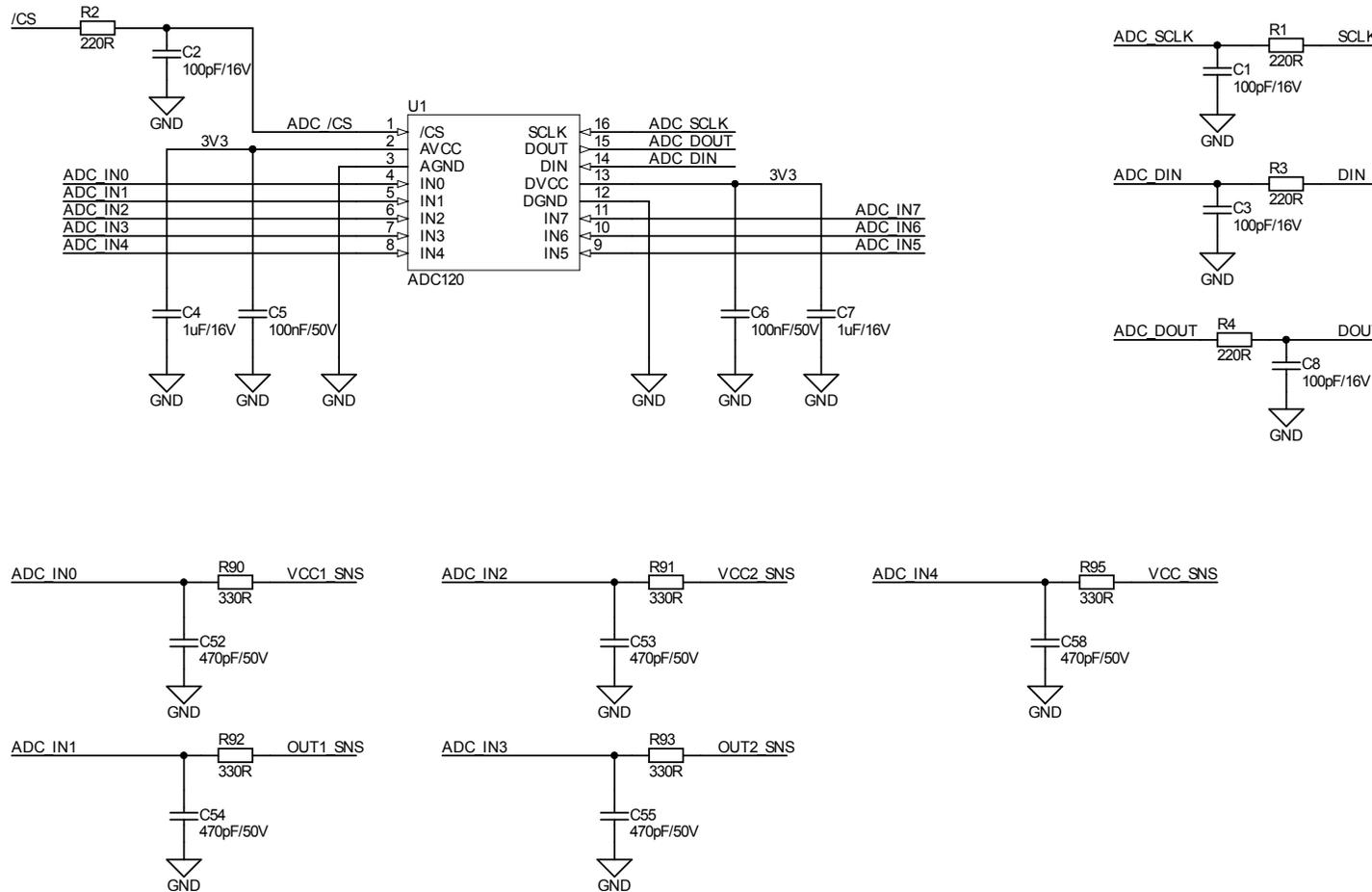
Figure 7. STEVAL-FSM01M1 circuit schematics (3 of 6)
