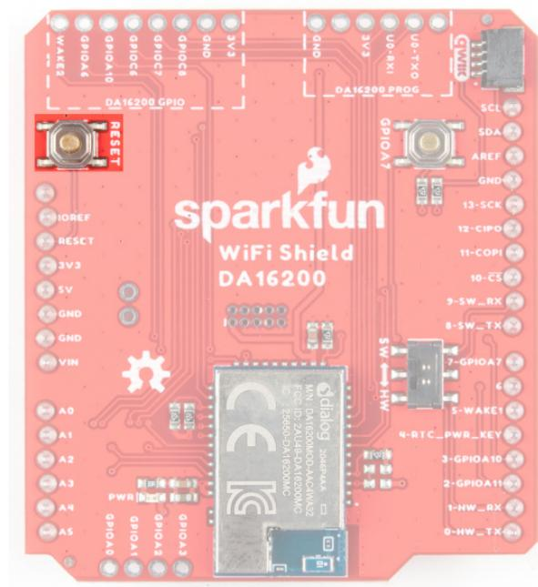
Pressing and holding GPIOA7 will perform a factory reset, which clears configurations that might have been saved to the module.
