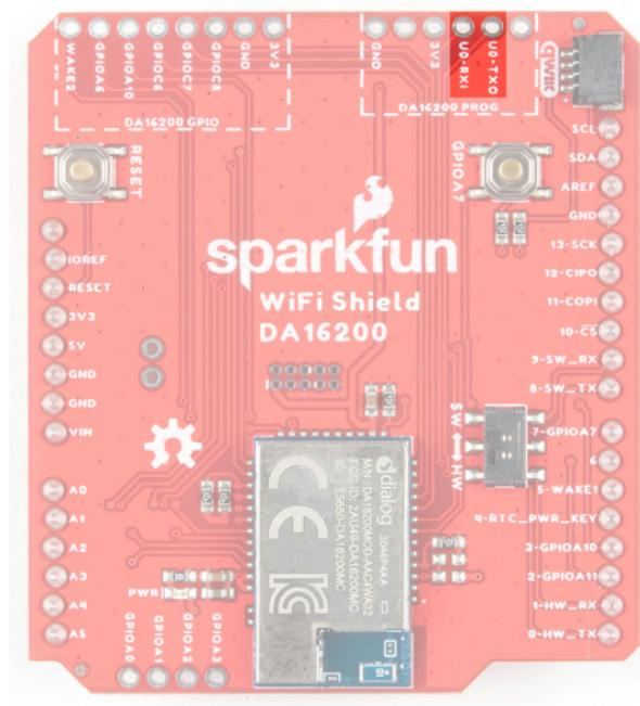
UART1 is used for sending AT commands and is routed through a switch to communicate through either the hardware UART pins D0/D1 for RX/TX, or software UART through D9/D8 for RX/TX.
