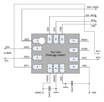
Primary: I2C Secondary: Auxiliary interface I2C (e.g. BMM150 sensor)
