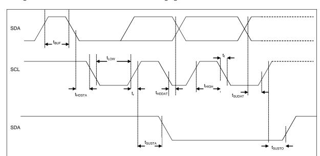
The figure below shows the definition of the I<sup>2</sup>C timings given in the above table:
