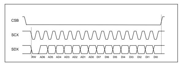
3-wire basic SPI write sequence (mode '11')
