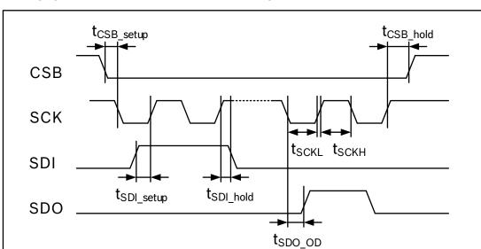
The following figure shows the definition of the SPI timings:
