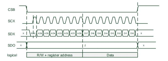
4-wire basic SPI write sequence (mode '00')
