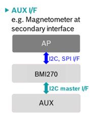
Figure 7: 9-DOF Solution w/ magnetometer (AUX) connected to the 2<sup>nd</sup> I/F
