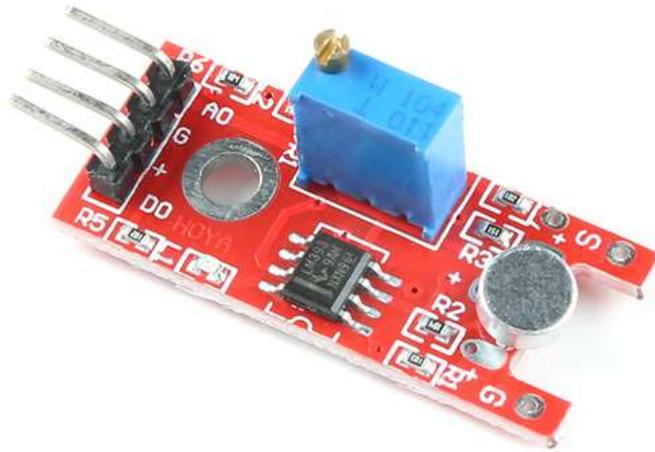
This is a 4-pin microphone voice sound sensor module based around the LM393 chip. It features an electric condenser microphone, single channel signal output with a low level output signal used for sound control light.
