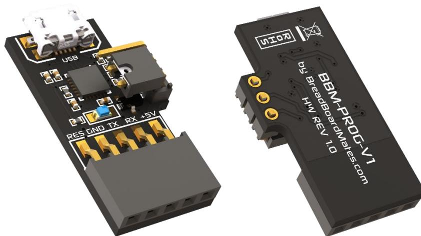
The BBM-PROG features a 3-pin jumper with shunt, which is present to change the way the programmer handles the Reset line, utilised by TED-96 and other devices.
