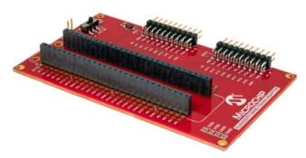
The Curiosity Nano Touch Adapter bridges from the Curiosity Nano MCU kits to the XPRO connected touch extension boards.
