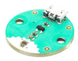
The Light module detects ambient light level. It's ideal for use in a weather station, keeping track of light levels in your greenhouse, or reminding you when you've left the lights on in your house.
