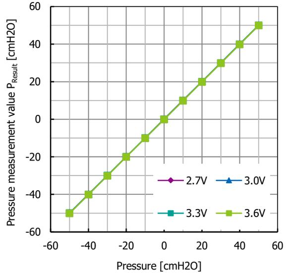
Fig. 23.2 Pressure measurement value  $P_{\text{Result}}$  supply voltage characteristic
