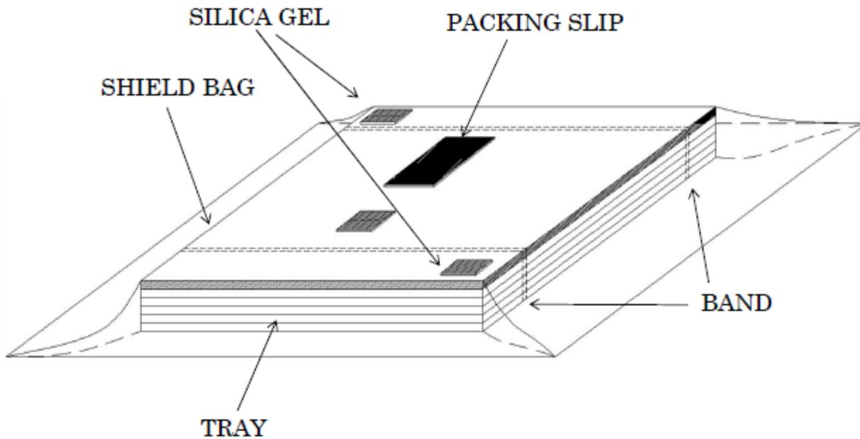
THESE 6 TRAYS WHICH ARE 5 TRAYS WITH PRODUCTS AND EMPTY TRAY AS LID ARE PILED UP. ALSO, THESE TRAYS ARE FIXED BY BAND. THESE ARE VACUUM-HEAT-SEALED TOGETHER WITH THE SILICA GEL.
