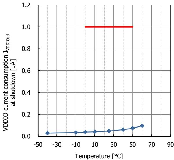
Fig. 22.7 VDDIO current consumption  $I_{VDDIOsd}$  at shutdown temperature characteristic
