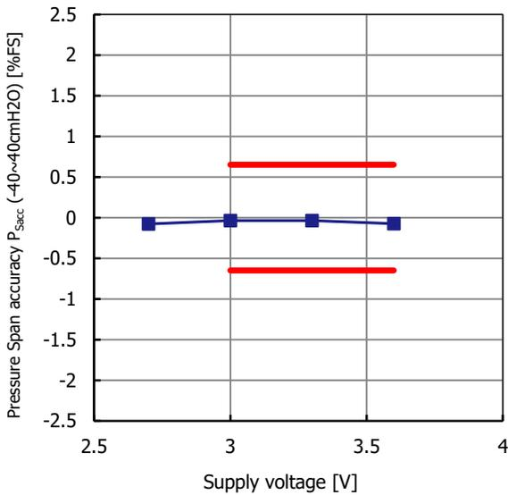
Fig. 23.7 Pressure Span accuracy  $P_{Sacc}$  supply voltage characteristic
