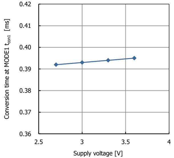
Fig. 22.10 Conversion time at MODE 1 supply voltage characteristic
