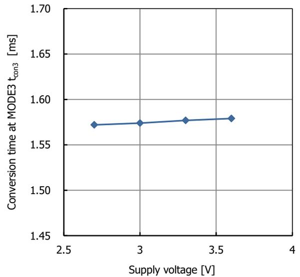
Fig. 22.14 Conversion time at MODE 3 supply voltage characteristic
