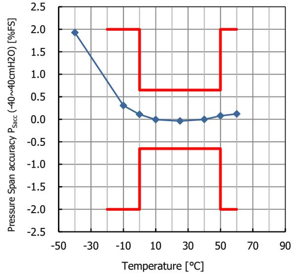
Fig. 23.6 Pressure Span accuracy  $P_{Sacc}$  temperature characteristic
