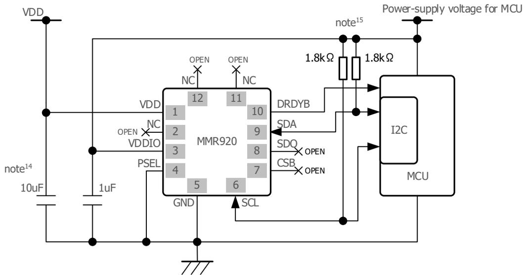
Fig. 21 Typical Electrical Connection (I2C)
