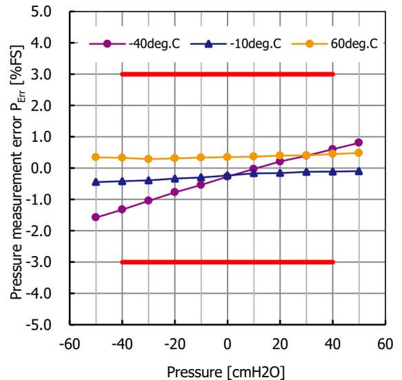
Fig. 23.4 Pressure measurement error  $P_{\text{Err}}$  temperature characteristic  $-40\sim 60^{\circ}\text{C}$
