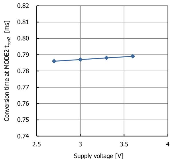
Fig. 22.12 Conversion time at MODE 2 supply voltage characteristic
