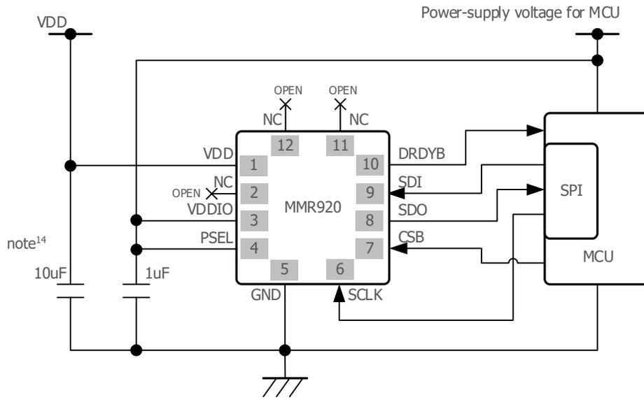
Fig. 20 Typical Electrical Connection (SPI)
