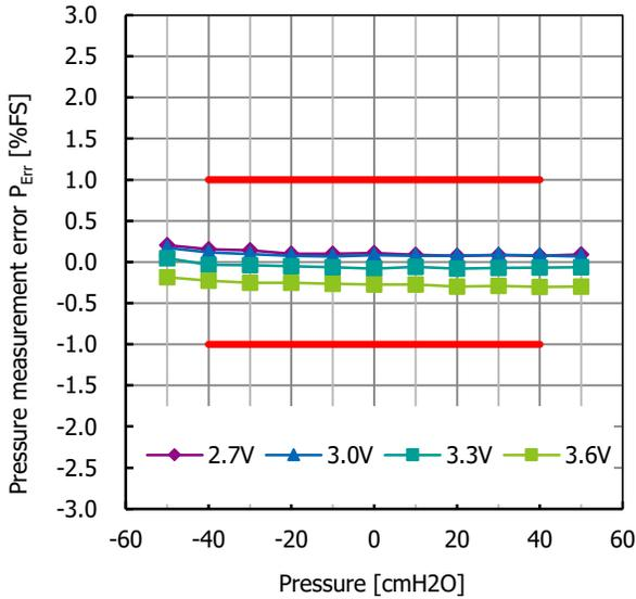
Fig. 23.5 Pressure measurement error  $P_{Err}$  supply voltage characteristic
