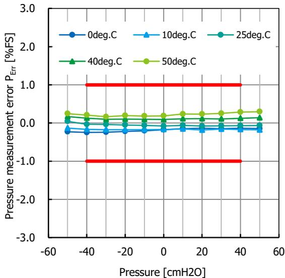
Fig. 23.3 Pressure measurement error  $P_{\text{Err}}$  temperature characteristic  $0\sim 50^{\circ}\text{C}$
