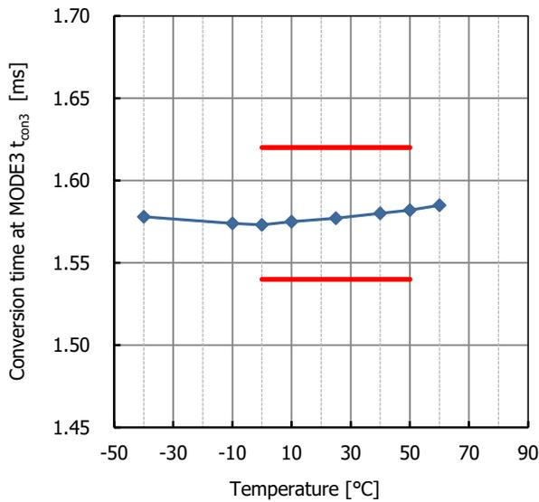
Fig. 22.13 Conversion time at MODE 3 temperature characteristic
