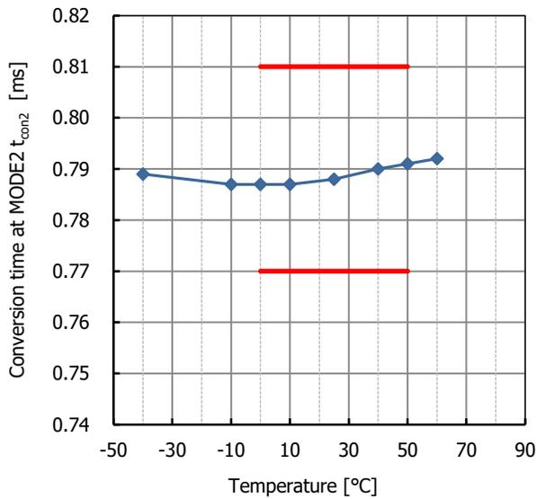
Fig. 22.11 Conversion time at MODE 2 temperature characteristic
