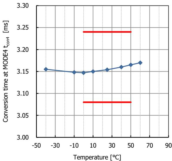
Fig. 22.15 Conversion time at MODE 4 temperature characteristic
