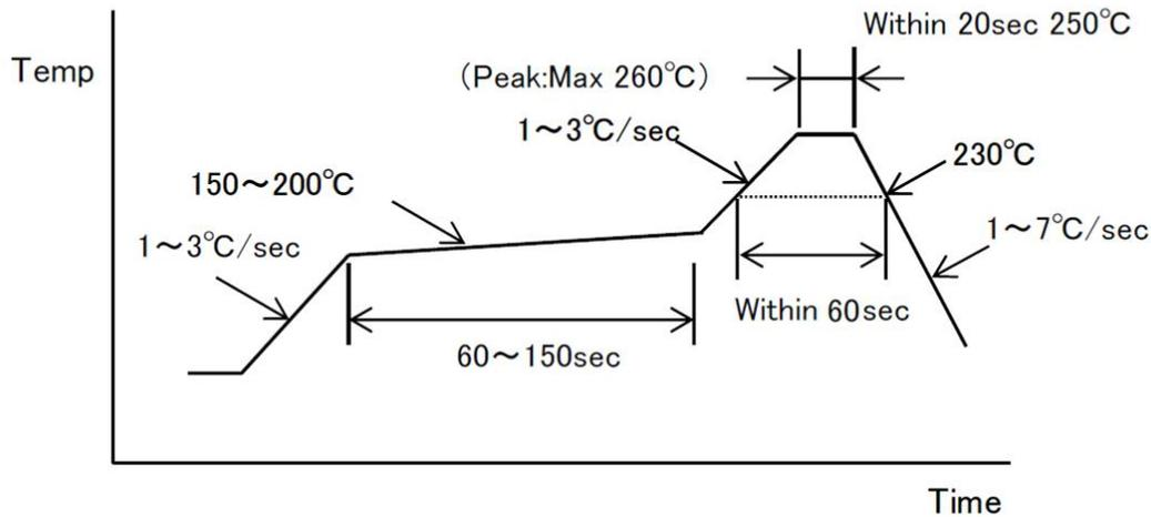
This profile gives recommended values, which are not guaranteed. For mounting the package, evaluate the profile with the equipment, conditions, and materials to be used.
