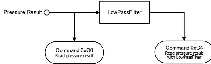
Fig. 9 Low Pass Filter Configuration
