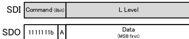
Fig. 14 SPI Write/Read format
