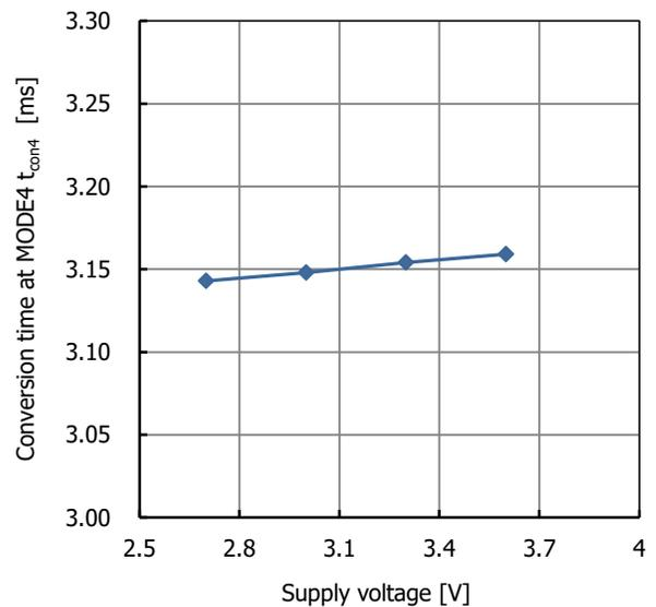
Fig. 22.16 Conversion time at MODE 4 supply voltage characteristic
