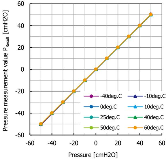
Fig. 23.1 Pressure measurement value  $P_{\text{Result}}$  temperature characteristic
