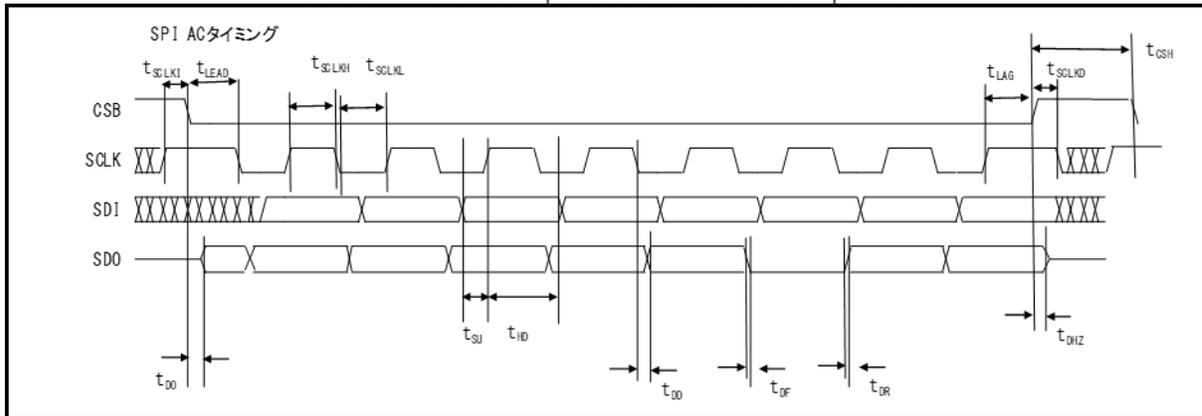
Fig. 11 SPI AC timing chart
