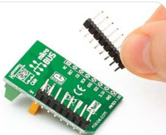
Turn the board upside down, so that bottom side is facing you upwards. Place shorter parts of the header pins in the both soldering pad locations.
