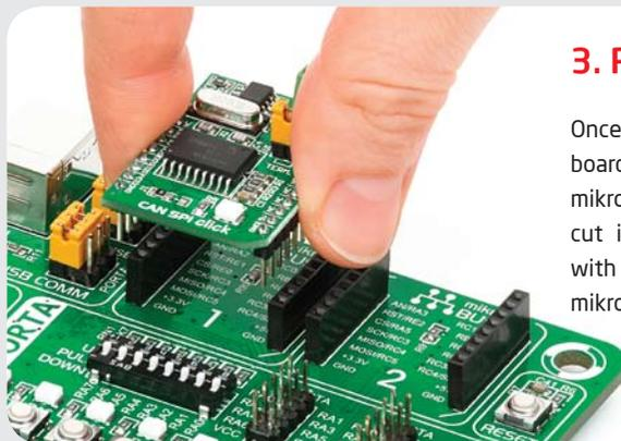
Once you have soldered the headers your board is ready to be placed into desired mikroBUS™ socket. Make sure to align the cut in the lower-right part of the board with the markings on the silkscreen at the mikroBUS™ socket. If all the pins are aligned correctly, push the board all the way into the socket.
