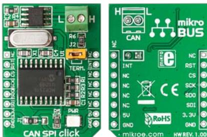
CAN SPI click 3.3V is an accessory board in **mikroBus™** form factor. It is the best solution for adding CAN connectivity to your microcontroller with SPI interface. Board features **SN65HVD230** CAN transceiver circuit which provides CAN serial communication physical layer in accordance with the ISO 11898 standard. It is designed for operation in especially-harsh environments, providing reliable solution. Board is designed to use 3.3V power supply only.
