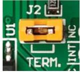
2. If the board is a node in the middle, jumper should be **removed**.
