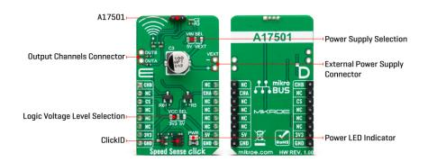
When properly back-biased, the sensor is intended for use with ring magnets or ferromagnetic targets. It poses a temperature-compensated amplifier, as well as a full-range ADC. Besides operating on 5V from the mikroBUS™ socket power rail, you can also add an external power supply over the VEXT connector from 4 up to 24V. The selection can be made over the VIN SEL.
