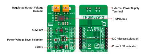
Step Down 11 Click uses a standard 2-wire interface of the AD5142A to allow the host MCU to set the output voltage, supporting 3MHz bandwidth. You can reset the digital potentiometer over the RST pin in case of need. The I2C address can be selected over the ADDR SEL jumpers (0 set by default). The power-good PG pin will be asserted if the output voltage is not within the specified window threshold. The EN pin is a precision enable input to the regulator.
