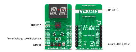
AlphaNum G 2 Click uses a standard 4-Wire SPI serial interface to communicate with the host MCU, supporting a clock frequency of up to 30MHz. A Blank BLK pin can turn all constant current outputs to OFF while initializing the grayscale PWM timing. This can be achieved by writing the High logic state on the Blank pin. You can also turn off every display separately, no matter the LED driver IC, over the CA1 and CA2 pins. Those pins control the common anode pins of the displays.
