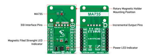
The MA735 uses integrated Hall devices to detect the magnetic field, while the angle is measured using MPS's proprietary Spinaxis™ method. This method is based on phase detection and digitizes the direction of the field directly, generating a sinusoidal signal with a phase that represents the angle of the field. The angle is obtained from a signal by a time-to-digital converter, and the digital number proportional to the magnetic field is delivered at a rate of 1MHz.
