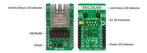
This Click board™ communicates with MCU through a standard SPI interface supporting the most common SPI mode, SPI Mode 0, with a maximum frequency of 20MHz. The operation of the ENC28J60 depends entirely on commands given by the host MCU over the SPI interface in the form of instructions of one or more bytes used to access the control memory and Ethernet buffer spaces. The entire buffer is 8 Kbytes, divided into separate receive and transmit buffer spaces used by the Ethernet controller.
