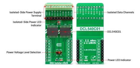
DIGI Isolator Click uses standard 4-Wire SPI serial interface lines, standard UART TX/RX interface lines, and two additional GP lines from the mikroBUS™ socket as an insulated extension, marked D2 and D1, respectively. The SPI and UART pins are labeled according to the standard interface markings. These eight lines go through the DCL540C01s to the terminals and headers, thus isolating the host MCU from the connected device.
