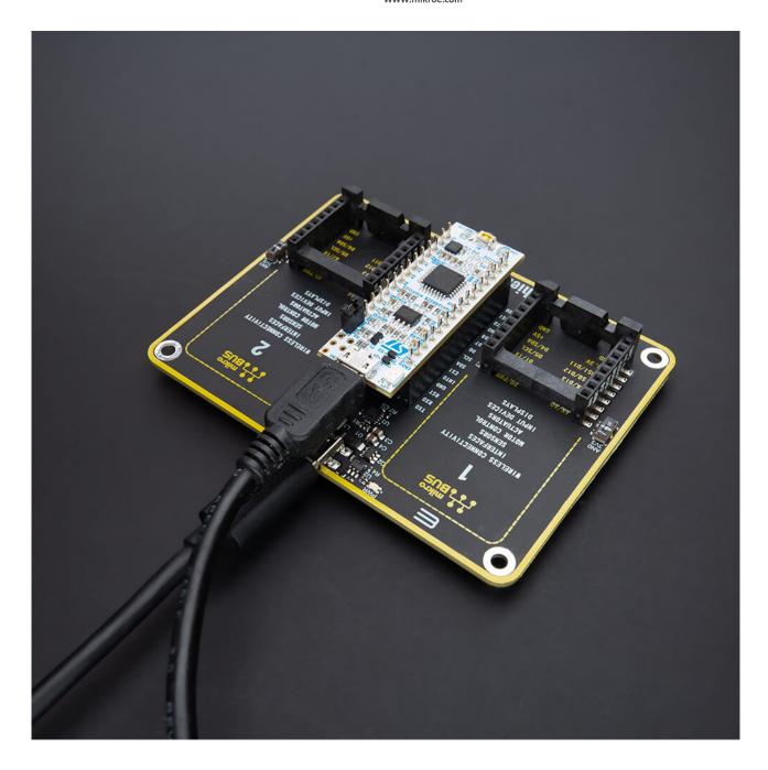
When the USB type C connector is connected to the Click Shield, and the other USB is connected to the STM32 Nucleo-32 board, the PWR diode will glow Cyan, and at this setup, the mikroBUS $^{\text{TM}}$  sockets are powered from the Type C connector.
