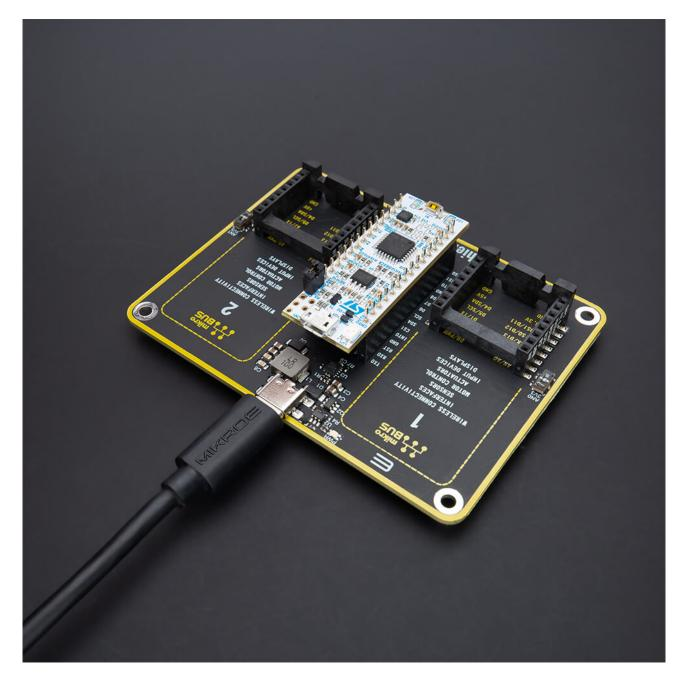
When the USB type C connector is connected to the Click Shield, the PWR diode will glow Blue, and at this setup, the connected STM32 Nucleo-32 baseboard and two mikroBUS $^{\text{m}}$  sockets will be powered from it.
