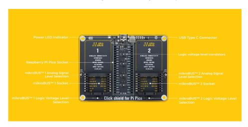
The Raspberry Pi Pico is based on the fast, efficient, and low-cost dual-core ARM Cortex-M0+ RP2040 microcontroller chip running at 133 MHz and sporting 264 KB of SRAM 2 MB of Flash memory, alongside Flash memory, crystal, power supplies, and decoupling, and USB connector. The majority of the RP2040 microcontroller pins are brought to the IO pins on the left and right edge of the board, which are then connected to two existing mikroBUS™ sockets.
