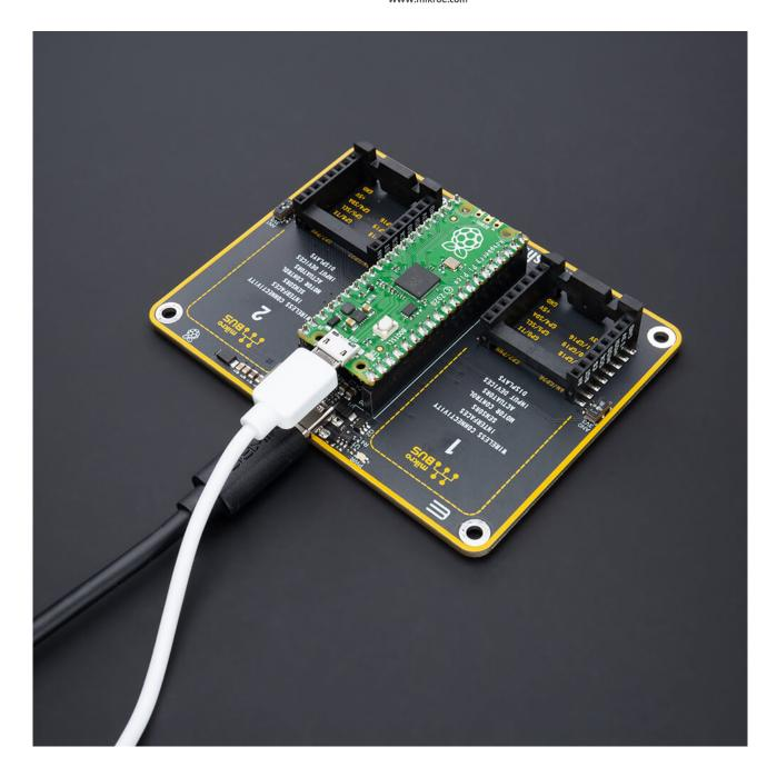
When the USB type C connector is connected to the Shield, and the other USB is connected to the Raspberry Pi Pico board, the PWR diode will glow Cyan, and at this setup, the mikroBUS $^{\text{m}}$  sockets are powered from the Type C connector.
