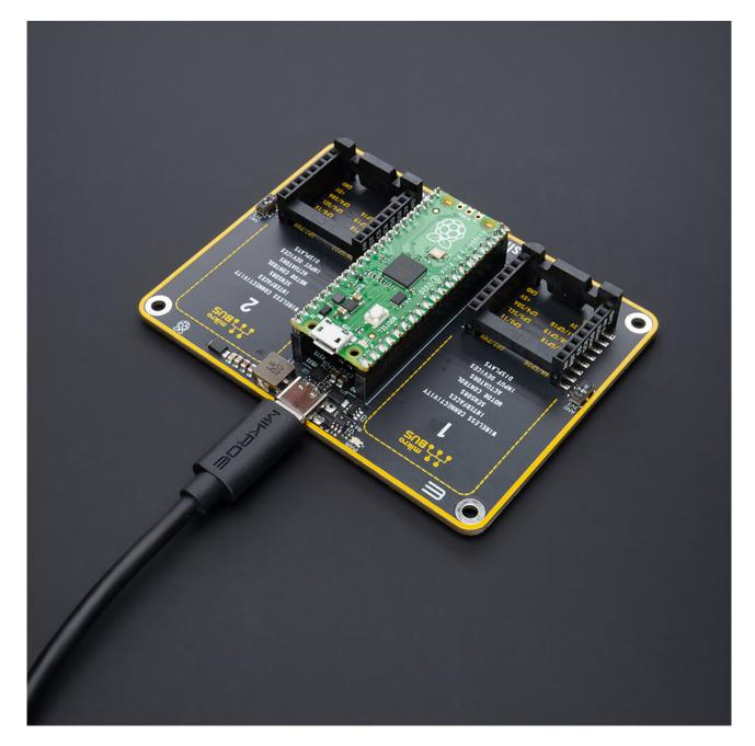
When the USB type C connector is connected to the Shield, the PWR diode will glow Blue, and at this setup, the connected Raspberry Pi Pico baseboard and two mikroBUS $^{\text{m}}$  sockets will be powered from it.
