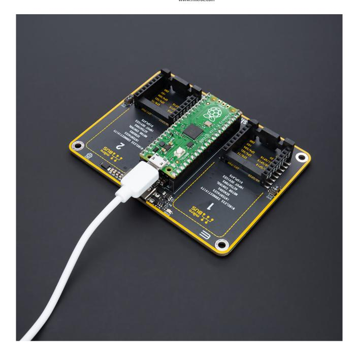
When the USB is connected to the Raspberry Pi Pico board, the PWR diode will glow Green, and at this setup, the Raspberry Pi Pico baseboard itself will be powered and provide power to the Shield, including two mikroBUS $^{\text{\tiny TM}}$  sockets.
