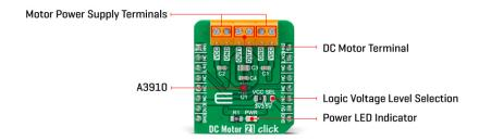
Using an integrated MOS switch improves braking action for the motor, compared to implementation with a simple clamp diode. Besides, it also features built-in protection such as crossover current and thermal shutdown protection, alongside "Sleep" Standby mode with zero drain-current.
