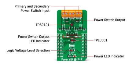
If one of the input power supplies were to fail, the system needs to automatically switchover to a backup power source without interrupting regular operation. When the 12V supply on IN1 drops below 7.6V, the device will automatically switch to the 5V auxiliary supply on IN2. When the 12V supply returns, it will become the output supply again. Furthermore, the voltage drop on the output should be minimal, providing the output with uninterrupted redundant power.
