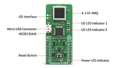
The Fingerprint 2 Click has stable performance and simple structure. The simplified functions for faster and easy development include fingerprint comparison, image scanning transmission, search, registered fingerprint storage and system unique internal code protection mechanism. The fingerprint comparison program can register at most 24 fingerprints, the comparison speed is fast and the correct rate is very high.
