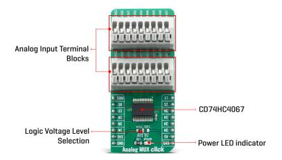
The CD74HC4067 IC is digitally controlled analog switch that utilize silicon-gate CMOS technology to achieve operating speeds similar to LSTTL, with the low power consumption of standard CMOS integrated circuits. The mentioned analog multiplexer/demultiplexer control analog voltages that may vary across the voltage supply range.
