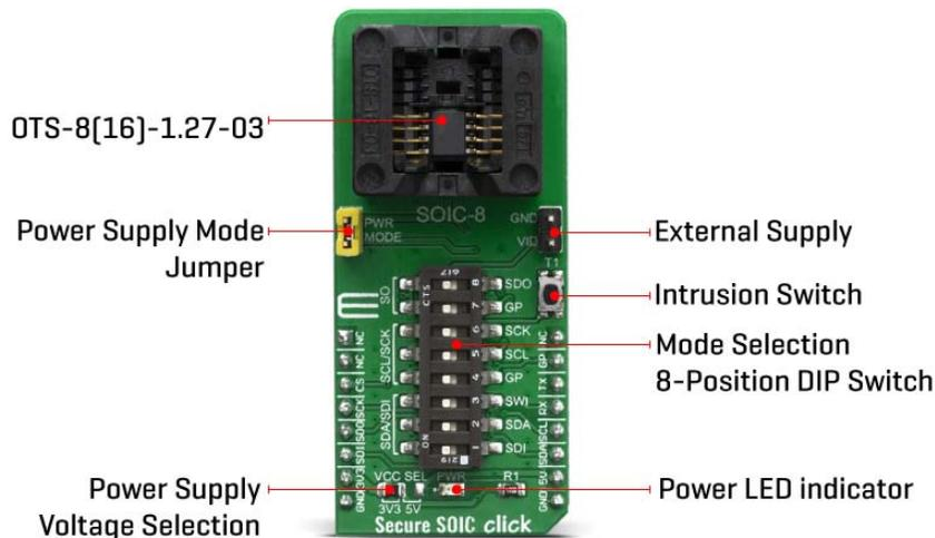
However, the Secure SOIC click is designed in a way that every IC from the CryptoAuthentication™ family from Microchip is fully supported with all of its features. Due to many different ICs and possibilities supported, the only way for achieving such a goal was to use the 8-positions DIP switch. That way, user is able to select the communication lines routed the way it is required for any application.
