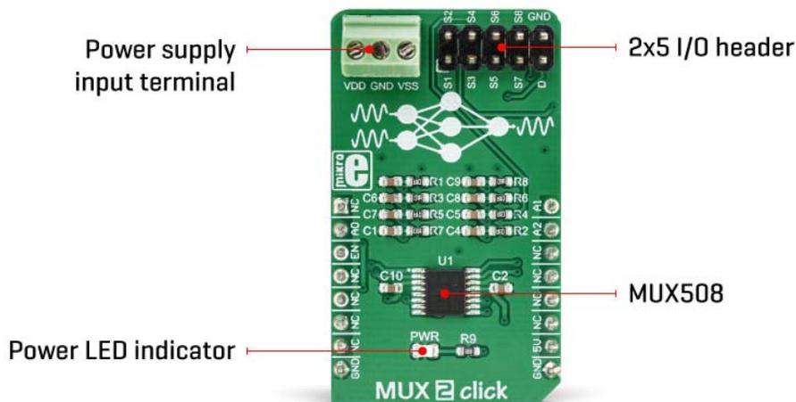
The MUX508 IC is targeted towards working with both bipolar and unipolar single-ended inputs. Each input is labeled as S1 to S8. When a specific channel is selected by using the A0 to A2 pins, it will be switched to the output pin, labeled as D. For the improved stability, each pin is equipped with the 100nF parallel capacitor and 100Ω series resistance. The input and the output signal pins are routed to the standard 2.54mm pitch 2x5 pins header on the Click board™.
