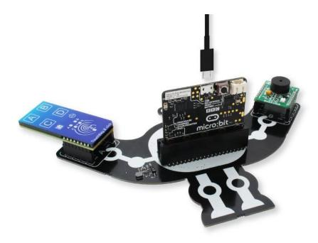
The **micro:bit Click adapter** is powered from the micro:bit itself. An 80pin edge connector allows easy installation to the micro:bit board. Due to the micro:bit symmetrical design, there is no wrong way of connecting. It can be plugged into the connector both ways, keeping it simple.
