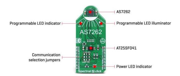
The measurements from the photo elements are digitized by the 16bit ADC converter and processed by the spectral\_ID engine. Besides the raw values of the six color elements, which can be read from the registers as 16bit integer values, the engine calculates all the calibrated values available on this device and outputs them as 32bit float values with an 8bit biased exponent and a 23bit fraction part. After the specified integration time, those
