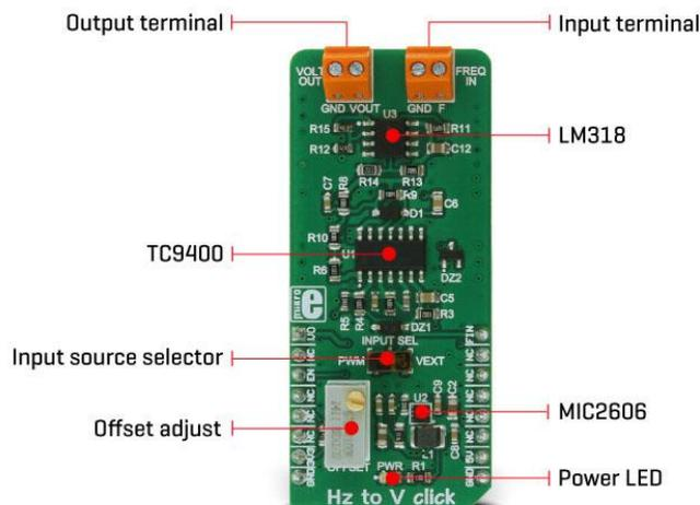
When Hz to V click is operated for the first time, it needs to be calibrated. The click is equipped with a variable resistor for the offset fine tuning. The following procedure should be followed to calibrate the device:
