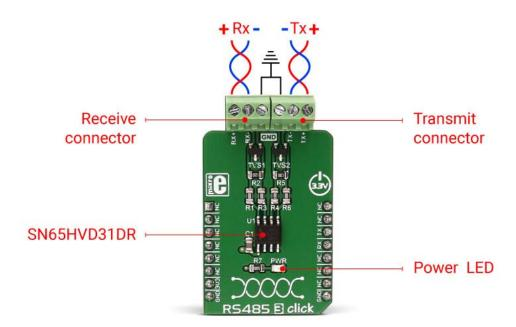
TX and RX pins should be used for connecting MCU UART interface. Two resistors (R2 and R5) should be unsoldered if using more than two clicks on the RS422/RS485 bus.
