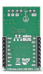
**Brushless 3 click** carries the DRV10983, a three-phase sensorless motor driver with integrated power MOSFETs. When an external power supply is applied, you can drive a brushless DC motor through the PWM pin, AN pin or I2C interface. It communicates with the target microcontroller over I2C interface, with the additional functionality provided by the following pins on the mikroBUS™ line: PWM, AN, INT, RST.
