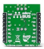
**Brushless 2 click** carries the DRV10964 BLDC motor controller with an integrated output stage from Texas Instruments. The click is designed to run on either 3.3V or 5V power supply. It communicates with the target microcontroller over the following pins on the mikroBUS<sup>TM</sup> line: AN, RST, CS, PWM, INT.
