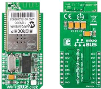
WiFi PLUS Click is an accessory board in **mikroBUS™** form factor. It's a compact solution for adding WiFi communication to your device. It features **MRF24WB0MA** - 2.4GHz, IEEE std. 802.11 - compliant module as well as **MCW1001** companion controller with on-board TCP/IP stack and 802.11 connection manager. WiFi PLUS click communicates with target board via UART interface. Board is designed to use 3.3V power supply only. It has an option to achieve low power consumption.
