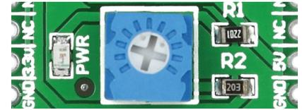
To calibrate CO click™ for optimum performance, use the on-board potentiometer to adjust the Load Resistance of the sensor circuit.
