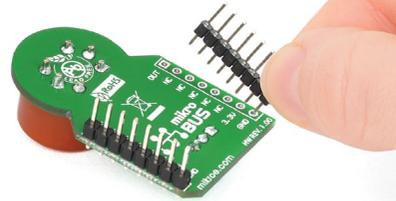
Turn the board upside down so that the bottom side is facing you upwards. Place shorter pins of the header into the appropriate soldering pads.
