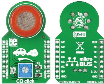
CO click™ is a simple solution for adding a high-sensitivity Carbon monoxide sensor to your design. The board features an MQ-7 sensor with a SnO<sub>2</sub> gas sensing layer, a calibration potentiometer, a **mikroBUS™** host socket, two jumpers and a power indicator LED. CO click™ communicates with the target board through mikroBUS™ AN (OUT) line. CO click™ is designed to use a 5V power supply only.
