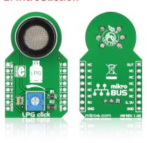
LPG click<sup>™</sup> is a simple solution for adding a high-sensitivity sensor for detecting liquefied petroleum gas leakage. The board features an **MQ-5** sensor with a SnO<sub>2</sub> gas sensing layer, a calibration potentiometer, a **mikroBUS**<sup>™</sup> host socket, two jumpers and a power indicator LED. LPG click<sup>™</sup> communicates with the target board through mikroBUS<sup>™</sup> AN (OUT) line. LPG click<sup>™</sup> is designed to use a 5V power supply only.
