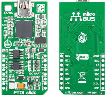
FTDI Click™ is an accessory board in **mikroBUS™** form factor. It's a compact and easy solution for adding USB to UART/SPI/I<sup>2</sup>C communication to your design. It features **FT2232H** dual high speed USB to multipurpose IC, DA converter as well as EEPROM. FTDI Click™ communicates with the target board microcontroller via **mikroBUS™** SPI (MOSI, MISO, SCK, CS), I<sup>2</sup>C (SDA, SCL), UART (Tx, Rx), RST, PWM, AN and INT lines. LED diode (GREEN) indicates the presence of power supply.
