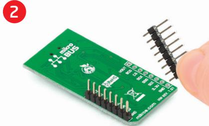
Turn the board upside down so that bottom side is facing you upwards. Place shorter parts of the header pins in both soldering pad locations.
