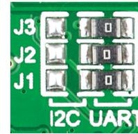
The FTDI Click™ board communicates with the main board microcontroller via I<sup>2</sup>C or UART interface depending on the position of the **J1**,
