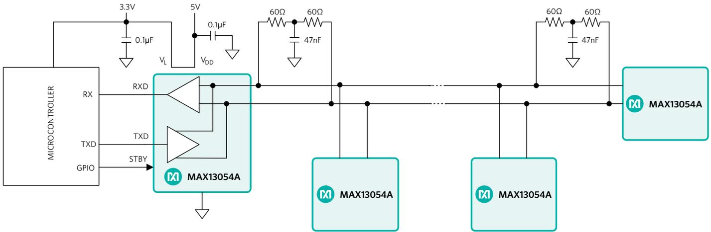
Figure 2. Multiple Receivers Connected to CAN Bus
