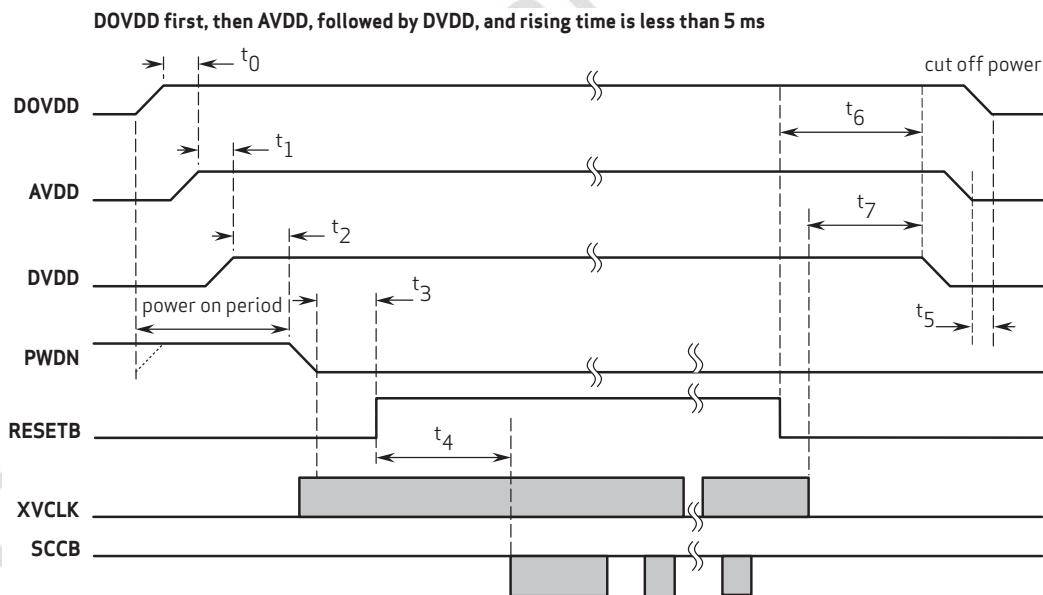
**note**  $t_0 \geq 0$  ms: delay from DOVDD stable to AVDD stable, it is recommended to power up AVDD shortly after DOVDD has been powered up
