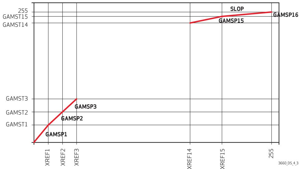
There are sixteen gamma control registers, including fifteen curve starting points and one highest slope. All of these control registers are configurable.
