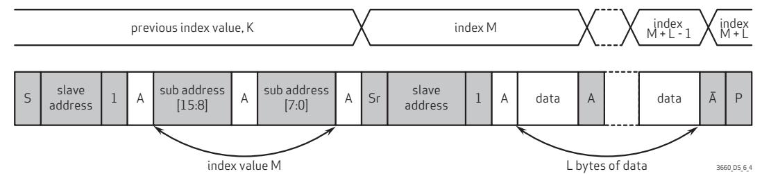
The sequential read from current location is similar to a sequential read from a random location. The only exception is that there is no dummy write operation, as shown in [figure 6-5](#). The master terminates the read operation by setting a negative acknowledge and stop condition.
