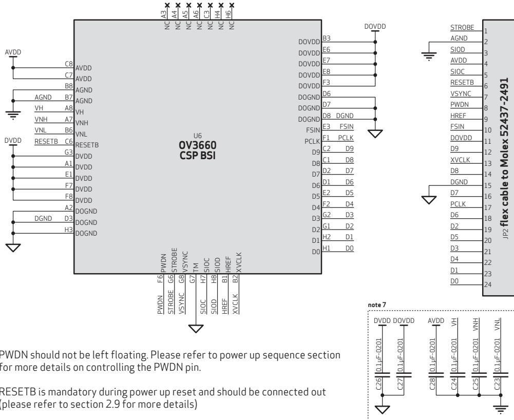
**note 1** PWDN should not be left floating. Please refer to power up sequence section for more details on controlling the PWDN pin.
