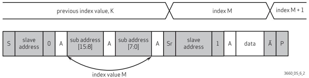
If the host addresses the camera with read operation directly without the dummy write operation, the camera responds by setting the data from last used sub-address to the SDA line as shown in **figure 6-3**. The master terminates the read operation by setting a negative acknowledge and stop condition.
