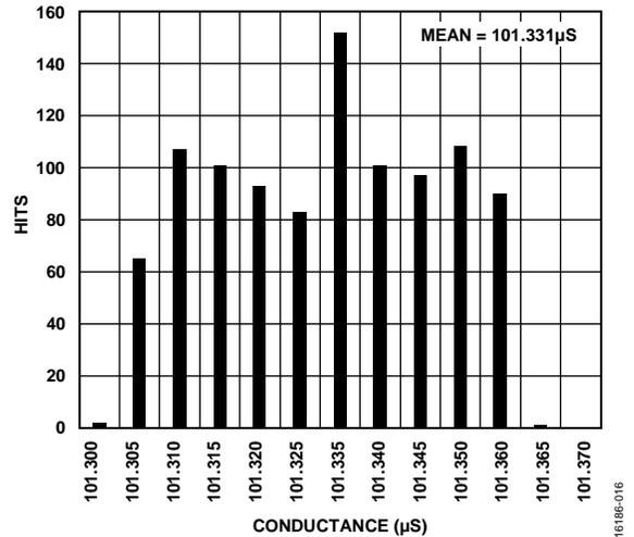
Figure 16. CN-0411 Noise Levels for a 100 μS Conductance
