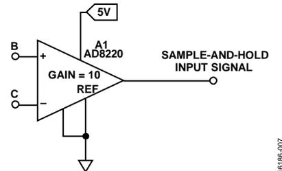
Figure 7. AD8220 Instrumentation Amplifier
