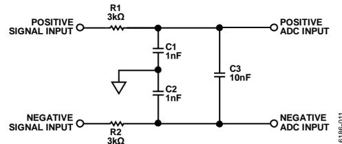
Figure 11. Typical RC Low-Pass Filter for Differential Inputs
