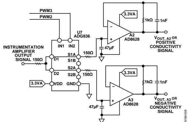
Figure 8. Sample-and-Hold Design Using ADG836 and AD8628
