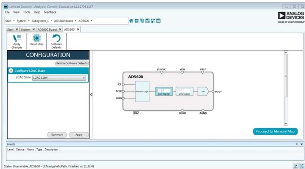
Figure 3. Chip Block Diagram of the AD5600
