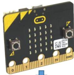
The edge connector has connections on only one side, so if the BBC micro:bit is inserted in reverse orientation, it will not work.
