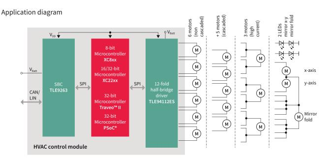
Example: The MOTIX™ TLE94112ES, 12-fold half-bridge, is designed to either drive 6 DC motors up to 0.9 A in parallel mode or 11 DC motors up to 0.9 A in cascaded mode or up to 3 DC motors up to 1.8 A by paralleling two outputs each. The device is sold in a PG-TSDSO-24 package and is pin and function compatible with the 6-, 8-, and 10-fold half-bridge of the TLE94xyz family.
