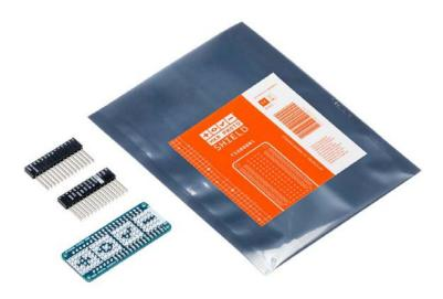
The MKR Proto Shield is a prototyping shield designed for your MKR board. This shield easily plugs onto your MKR using its provided female/male headers, and offers a duplicate breakout for each pin on the board along with many solderable throughholes on a standard 0.1" grid (2.54mm).
