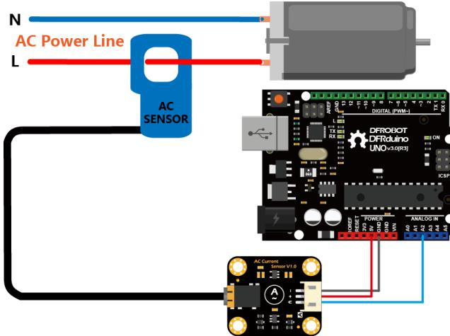
⚠ The AC transformer probe can only clamp to one of the AC wire. **It cannot be clamped both at the same time!**
