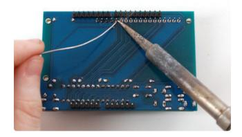
Flip over the shield and place it flat on the table so the long leads of the header stick out.
