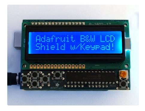
The shield is designed for 'classic' Arduino-shaped boards such as the Uno, Metro, etc. But it will also fit "Mega" sized boards because the I2C pins are labeled SCL/SDA.
