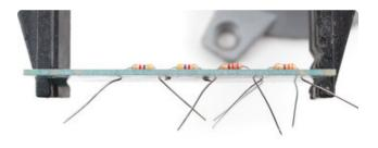
Make sure the resistors all sit nice and flat against the PCB.
