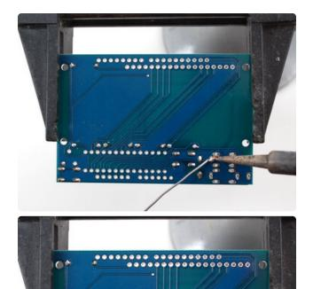
Solder each leg, taking care not to accidentally 'short' two button legs together. The ones for the directional pads are very close!
