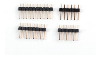
Take a stick of 36 pin header and break off a 10 pin piece, an 8 pin piece and two 6 pin pieces.
