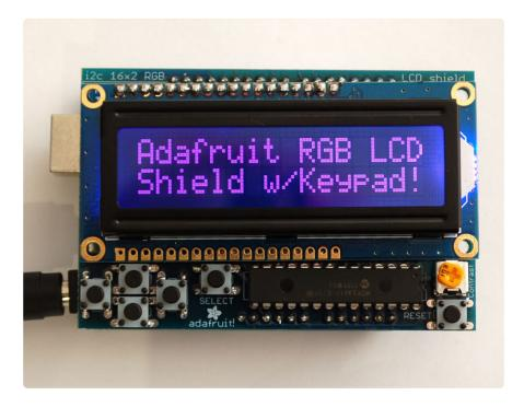
With this in mind, we wanted to make it easier for people to get these LCD into their projects. So we devised a shield that lets you control a 16x2 Character LCD, up to 3 backlight pins AND 5 keypad pins using only the two I2C pins on the Arduino! The best part is you don't really lose those two pins either, since you can use I2C-based sensors, real-time clocks, etc. and have them share the I2C bus. This is a super slick way to add a display without all the wiring hassle.
