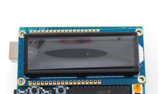
Next, check if you have an RGB LCD (with 18 pins) or a Monochrome display (not RGB, with 16 pins).
