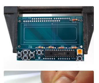
We're nearly done! Now we will place the I2C port expander chip. Double check that it has the MCP23017-E/SP marking on it. This is a 16-pin expander chip, that uses the i2c bus. That means you can send it commands using the i2c pins on an Arduino and control 16 more digital pins! 5 of those pins go to the buttons, 6 go to the LCD control and 3 are used for the backlight (the remaining 2 are unused).
