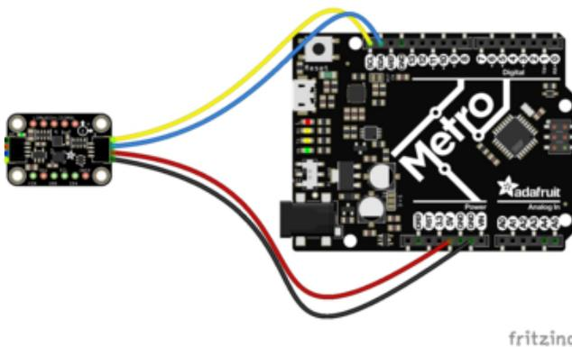
Board 5V to sensor VIN (red wire)
