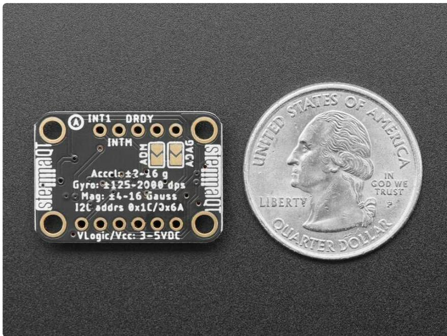
To make getting started fast and easy, we placed the sensors on a compact breakout board with voltage regulation and level-shifted inputs. That way you can use them with 3V or 5V power/logic devices without worry. To make usage simple, we expose only the I2C interface and some interrupt pins from each chip. The breakout comes fully assembled and tested, with some extra header so you can use it on a breadboard. Four mounting holes make for a secure connection.
