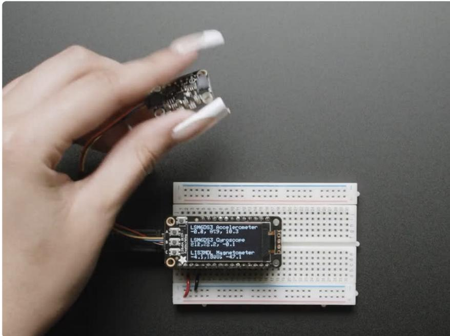
Add high-quality motion, direction, and orientation sensing to your Arduino project with this all-in-one 9 Degree of Freedom (9-DoF) sensor with sensors from ST. This little breakout contains two chips that sit side-by-side to provide 9 degrees of full-motion data.
