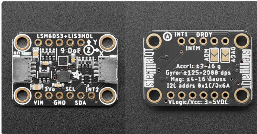
The default I2C address for the LSM6DS3 accelerometer is **0x6A**.
