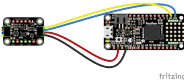
Board 3V to sensor VIN (red wire)
