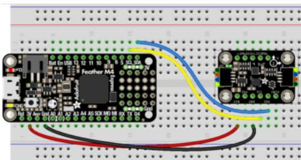
Board 3V to sensor VIN (red wire)
