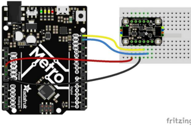
Board 5V to sensor VIN (red wire)
