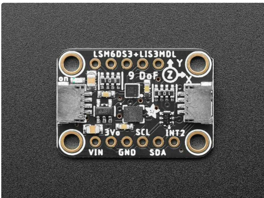
This chip is very similar to the now-discontinued LSM6DS33, a great entry-level IMU. As part of the illustrious LSM6DS family, it's well-established and well-supported, and this chip even has better performance! Note it is not firmware-compatible with the 'DS33, so you will need to recompile code (e.g our Arduino and Python libraries support the whole family but you do have to indicate which exact chip you're using)
