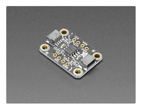
Usage is easy - you get power/ground/clock/data breakout pads for each side as well as a matching STEMMA QT connector. **Unlike our other QT boards, the two sides are obviously electrically isolated, which means each half must be powered!** Check that the green LED is lit on both sides. Now send data over I2C and you're good to go. We have 10K pullups on each side, from the I2C pins to the matching VCC for that side.
