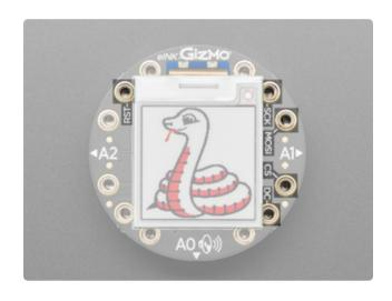
The display used on the E-lnk Gizmo is a 1.54" tri-color e-lnk display.
